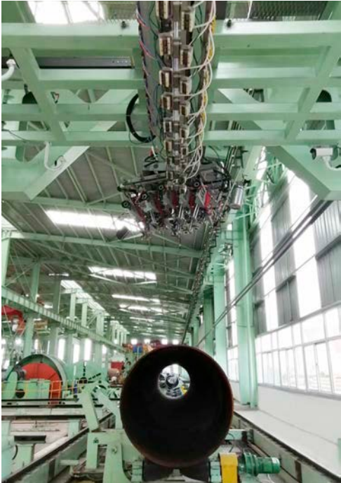
02 超声波连续探伤 Continuous Ultrasonic Inspection
